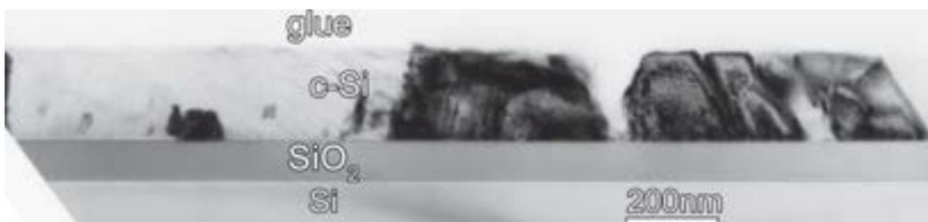
Figure 2: Bright Field TEM image showing the structure of the sample F2001
