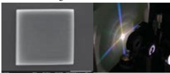
Figure 1: A 500 nm period photonic crystal structure (left) and the diffraction pattern of the same structure (right)
