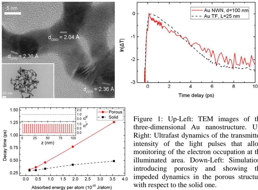
Figure 1: Up-Left: TEM images of the three-dimensional Au nanostructure. Up-Right: Ultrafast dynamics of the transmitted intensity of the light pulses that allow monitoring of the electron occupation at the illuminated area. Down-Left: Simulations introducing porosity and showing the impeded dynamics in the porous structure with respect to the solid one.
