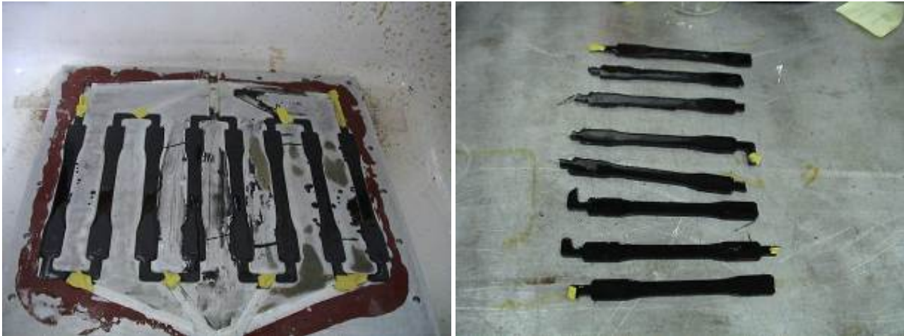
Figure 1: Photographs of the (a) metallic mould that tensile specimens were produced and (b) demoulded tensile specimens.
