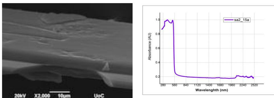
**Figure 1.** (a) Representative SEM image of the organic inorganic  $(C_6H_5CH_3NH_3)PbI_3$  perovskite and (b) the corresponding UV-Vis spectrum.
