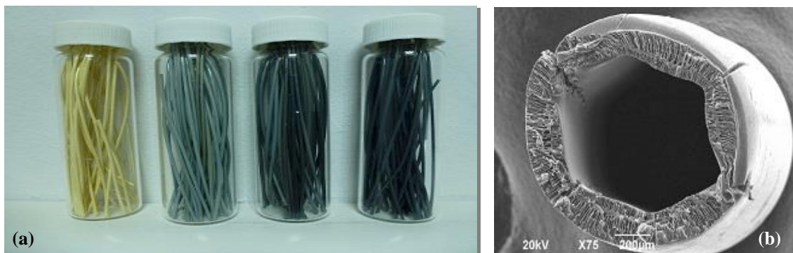
Figure 1: (a) Macro-photograph of the produced hollow fibers with different MWCNTs concentration (from left to right: MMHFM with 0, 1, 2 and 4 % fillers' concentration) and (b) SEM of the cross-section of the 0% MWCNTs hollow fiber [2]
