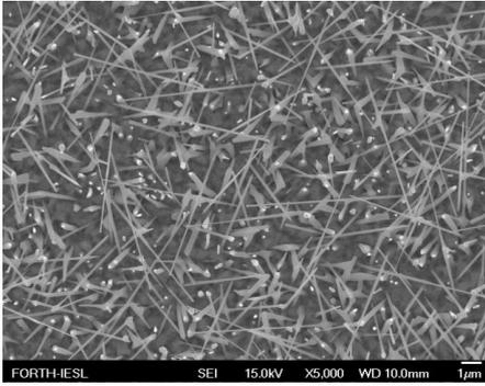
Figure 1: Top view SEM image of a NW Sample.
