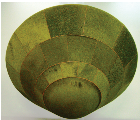
Figure 1. The Heat-shield demonstrator tested and built for FP7/RastasSpear
