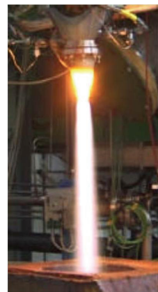
Figure 2. A satellite rocket combustion chamber (glowing) undergoing static tests
