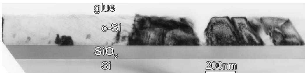
Figure 2: Bright Field TEM image showing the structure of the sample F2001
