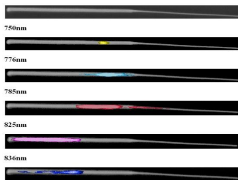
Figure 1: CL measurements in a single NW depicting the emission from different regions.
